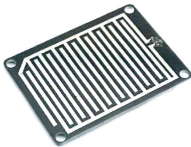
Figure 2.2.2 Water Level Sensor
