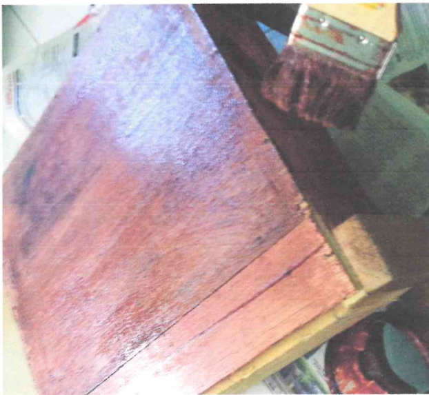
FIGURE 20: (brush the paint on it)
