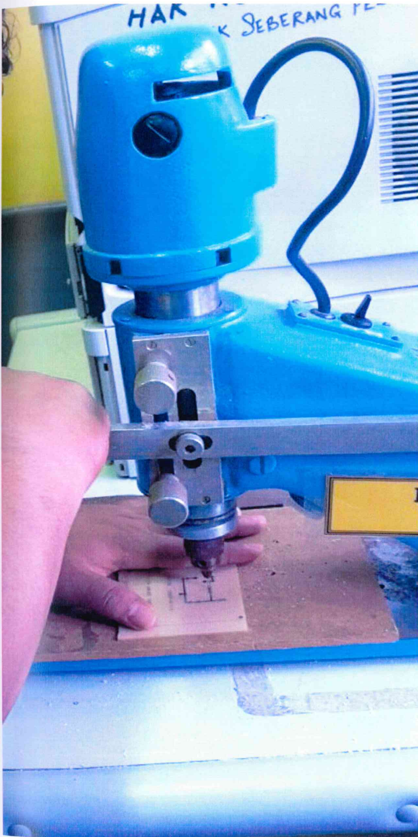
9.2 Figure show process of drilling the board
