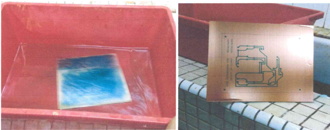
Figure 3.7.3: Process wash with copper water Figure 3.7.3: After wash with Copper water
