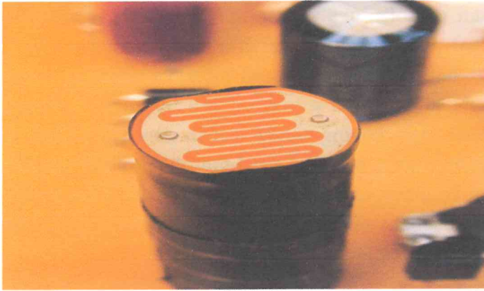
Figure 2.5: LDR (light dependent resistor)
