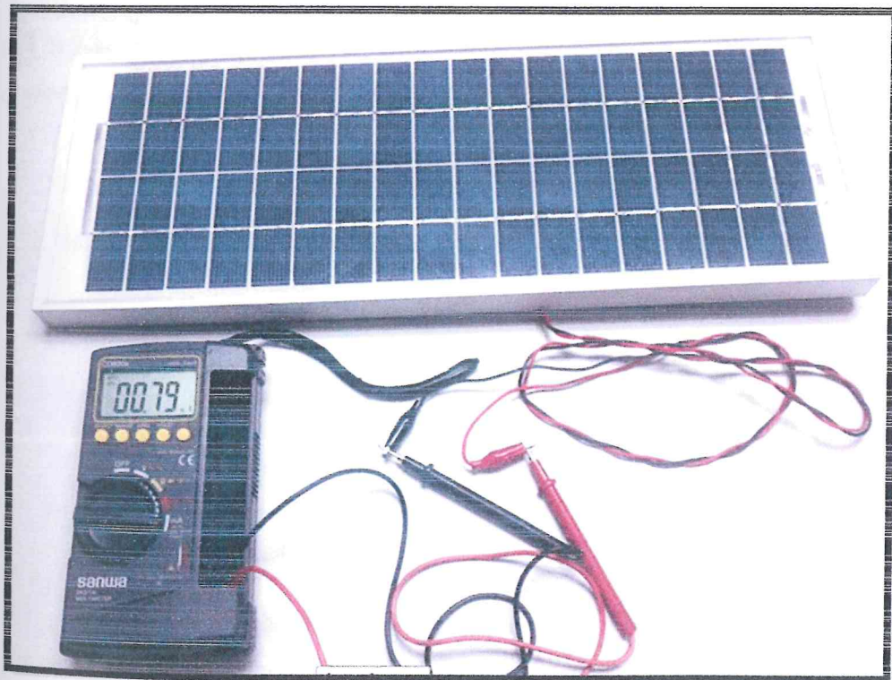
Figure 4.2 : Short Circuit Current Test
