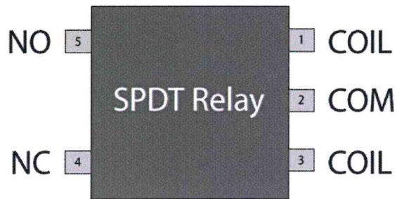
Figure 2.2.6.2 : Pin Diagram SPDT Relay
