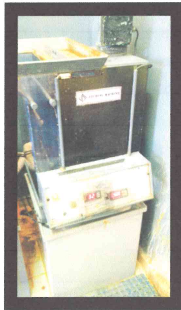
Figure 3.4.1.2 : Remove copper from board with ferric chloride
