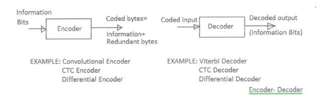
Decoder module utilizes redundant information present in the corrupt received vector to recover the original information bits which might have been transmitted.
