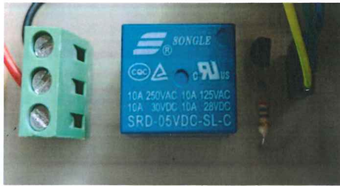
Figure 2.4 2(c) Relay on PCB Board
