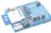
Adafruit Datalogging Shield with a Secure Digital (SD) card slot and real-time clock (RTC) chip
