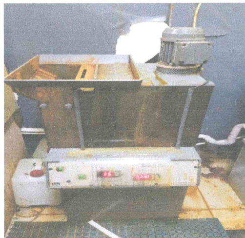
Figure 3.2.3.3 :Removal Of Copper On Etching Board
