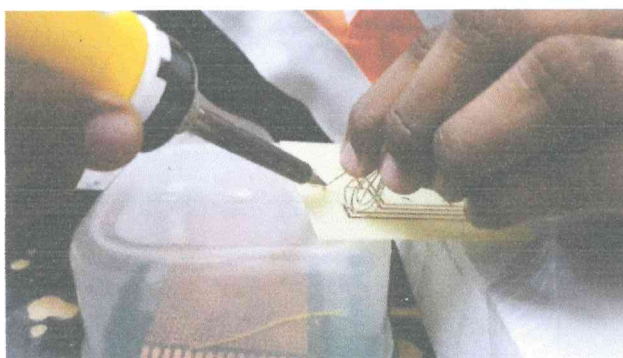
Figure 3.2.3.6 :Soldering Of Components On Etching Board
